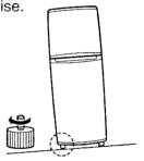
EN: When the refrigerator leans to the right, turn the right front foot counterclockwise.
