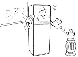
EN: Allow a 50mm space between the refrigerator and the wall.
