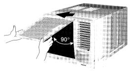
Pull up the front intake grille about  $90^{\circ}$  and slide it slightly to the left to unhook the tabs.
