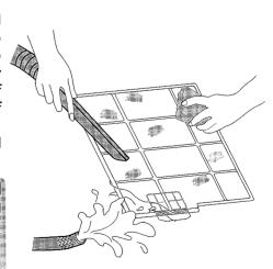
**NOTE:** Do not dry the front panel or the air filter in direct sunlight. (Exposure to direct sunlight may discolor or deform the panel.)
